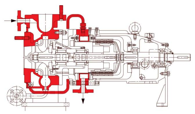
Pump with heating jacket, type PRM b
