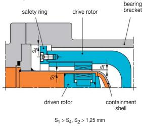
Due to the radial clearance  $S_2 > 1,25$  mm the pumps can handle non-metallic (non-ferrous) particles in the fluid up to 1,0 mm.
