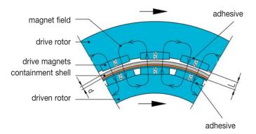
The couplings are designed to transmit rated motor power up to 220 kW (295 hp) at 2900 rpm, respectively 260 kW (348 hp) at 3500 rpm.
