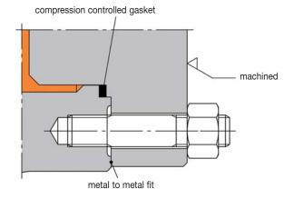
Pump flanges are full or spot faced on the back and designed for through-bolting.
