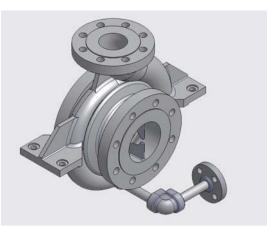
The pump casing forms - together with the containment shell - the pressure retaining pump part. Maximum allowable pressure at PT is determined by the shell design and the material. The pump casing has metal-to-metal fits with confined compression controlled gaskets.
