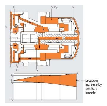
The cooling flow is led from the discharge side behind the impeller into the chamber between the slide bearings and through the pump shaft via the auxiliary impeller again to the discharge side. This design pressurizes the slide bearings and the containment shell with nearly the full discharge pressure and the product remains stable in this area.
